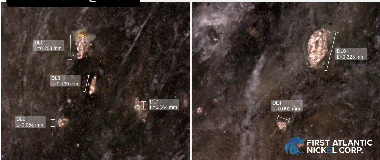
Figure 3: Drill core RPM DDH004 at 401 meters depth. Top image: Abundant, visibly disseminated awaruite grains (typically 50-100 microns, with some up to 323 microns). Bottom image: Awaruite grains from RPM DDH004 at 401 meters depth under a microscope, showing grains well above 10 micron size required for effective magnetic separation and recovery.
